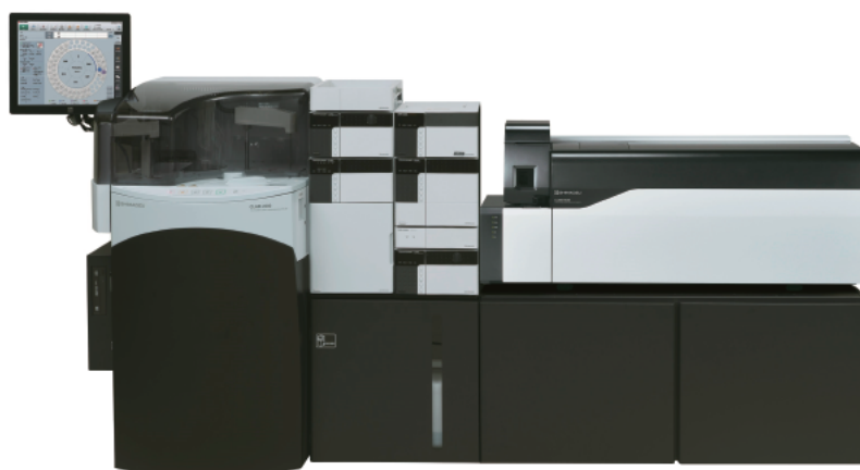
Figure 1: CLAM-2000 online with Nexera X2 system and LCMS-8050 triple quadrupole mass spectrometer.
